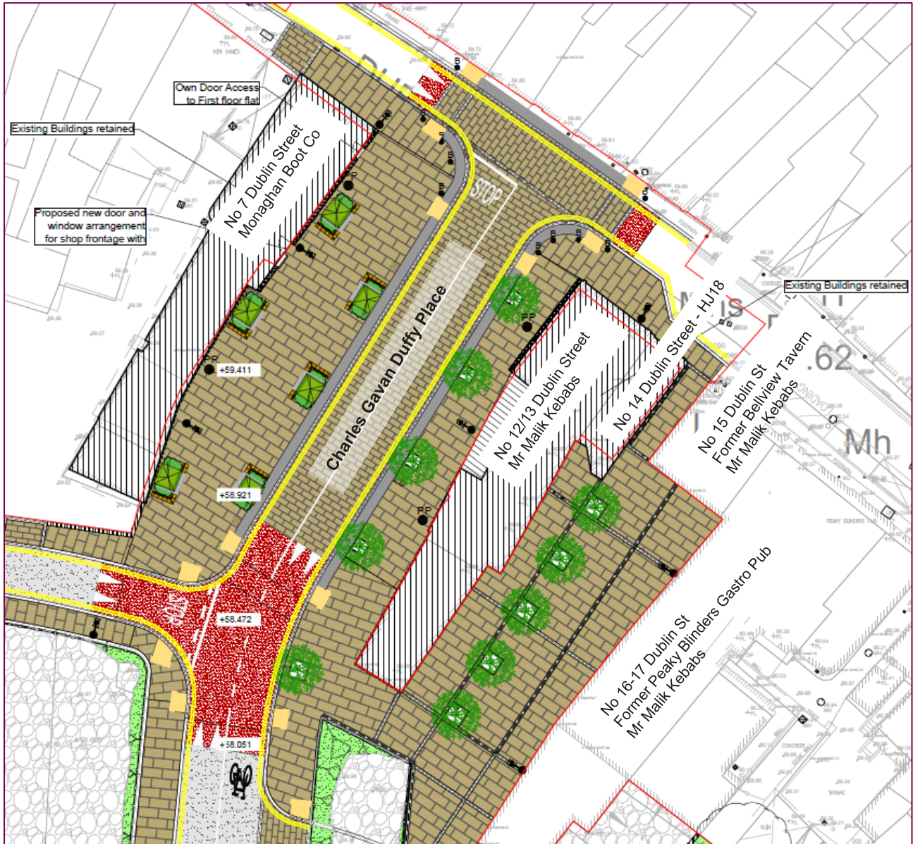
Figure 2.8: Proposed General Arrangement of Charles Gavan Duffy Place / Dublin Street
