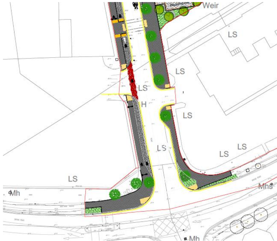
Figure 9.13 – N54 Macartan Road / Farney Road proposed layout
