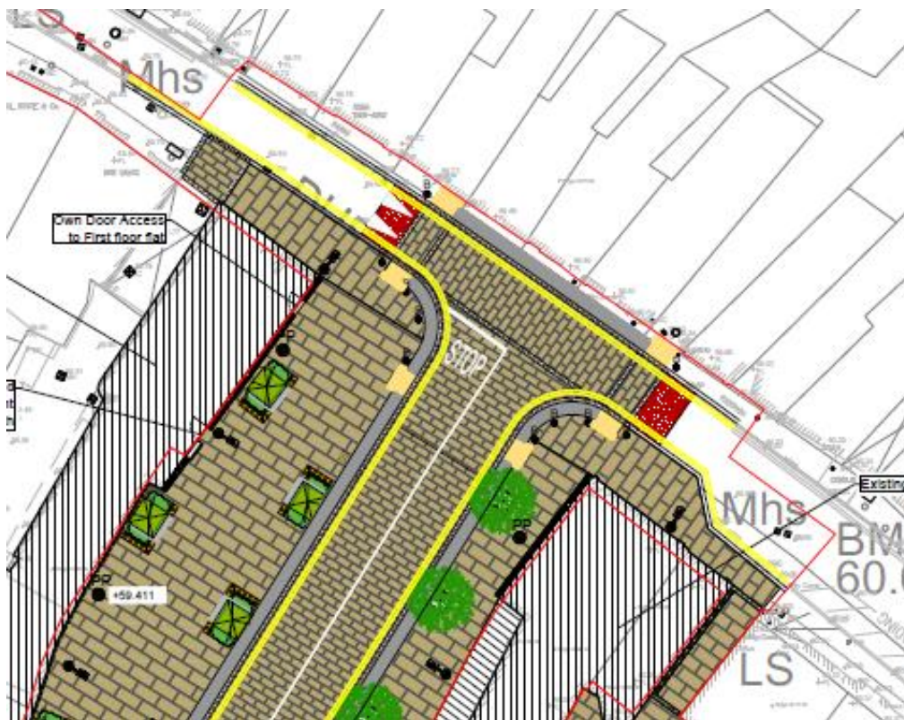
Figure 9.12 – Dublin Street / Charles Gavan Duffy Place proposed layout
